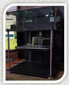
The DST-200 is a surface tensiometer for measurement of fluid's surface tension force based on du nouy method.
