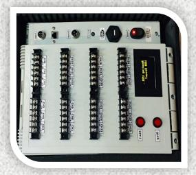
The ART-SR2424 is a multi-channel seismic recorder for reflection, refraction and exploration seismic investigations.
