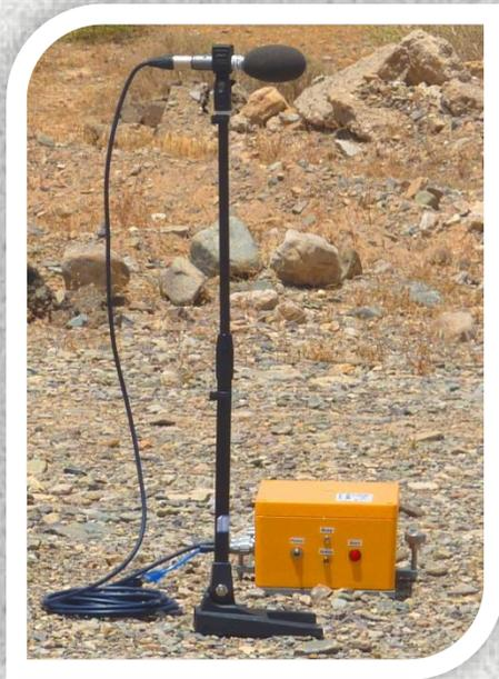
The BLS244 is a blast recorder which records both triaxial velocity and air blast pressure due to explosion.
